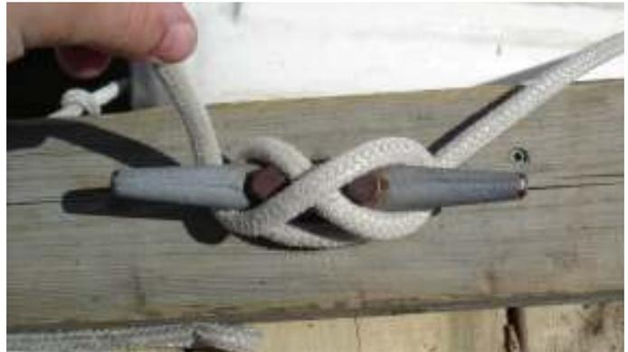
Step 3: Now comes the tricky part. To make sure that the painter stays securely tied to the horn cleat, you must keep crossing it from one “horn” to the next but this time you must make a loop out of the painter before putting it around the “horn”. Look carefully the image below.
