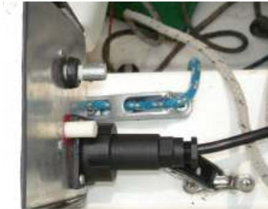
For the “sip n’ puff” system, the straws plug into the two white extremities at the front of the autohelm. The picture above illustrates the two white extremities. Some boats use an external sip n’ puff connector, which is simply a small box with similar connections.
